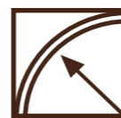
Standard radius 200 mm (Reverse bends 150 mm)
