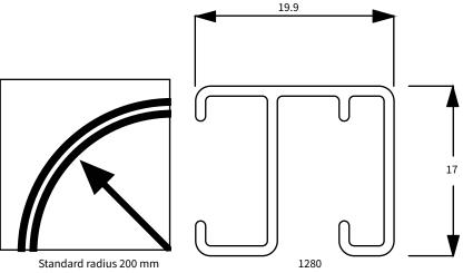
The standard radius is recommended for optimal operation. The minimum possible radius is 150 mm.
