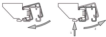
Installation: Roll track onto bracket in direction indicated Removal: 1. Press to release 2. Rotate forward for removal
